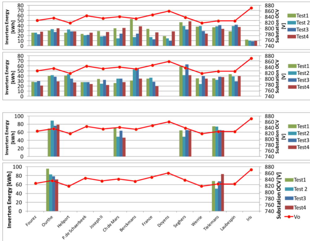
Figure 19 : Incremental approach for selecting the highest-potential substations, VUB – R. Barrero
