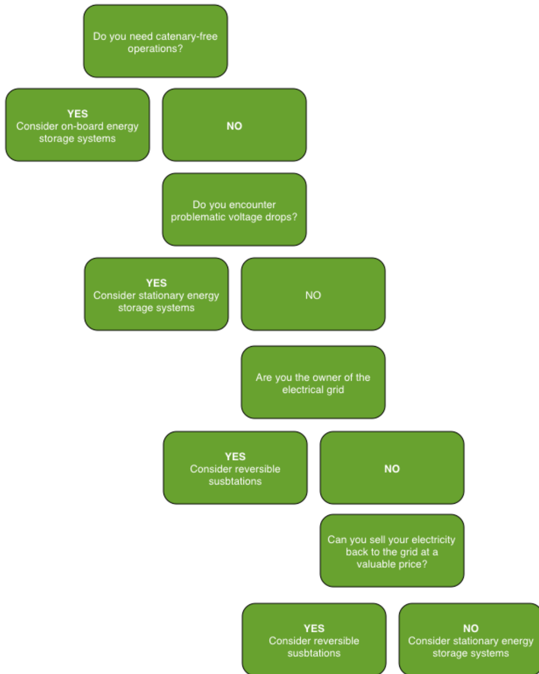
Figure 9 : Quick scan for identifying suitable braking energy recovery applications, Ticket to Kyoto
