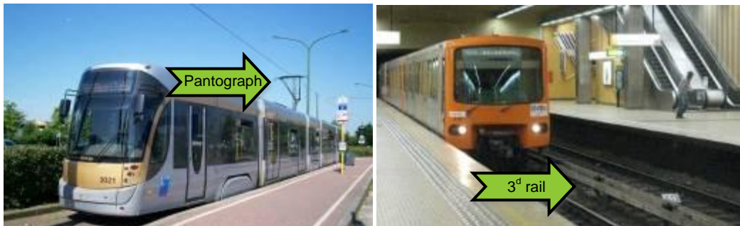
Figure 1 : View of a pantograph (tram network) and a third rail (metro network)
