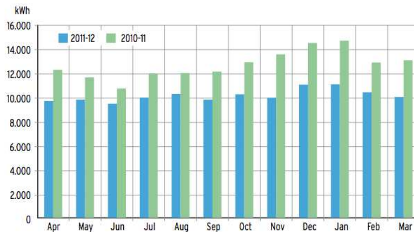
Figure 32 : Energy savings with LEDs at Hyde Bus Station
